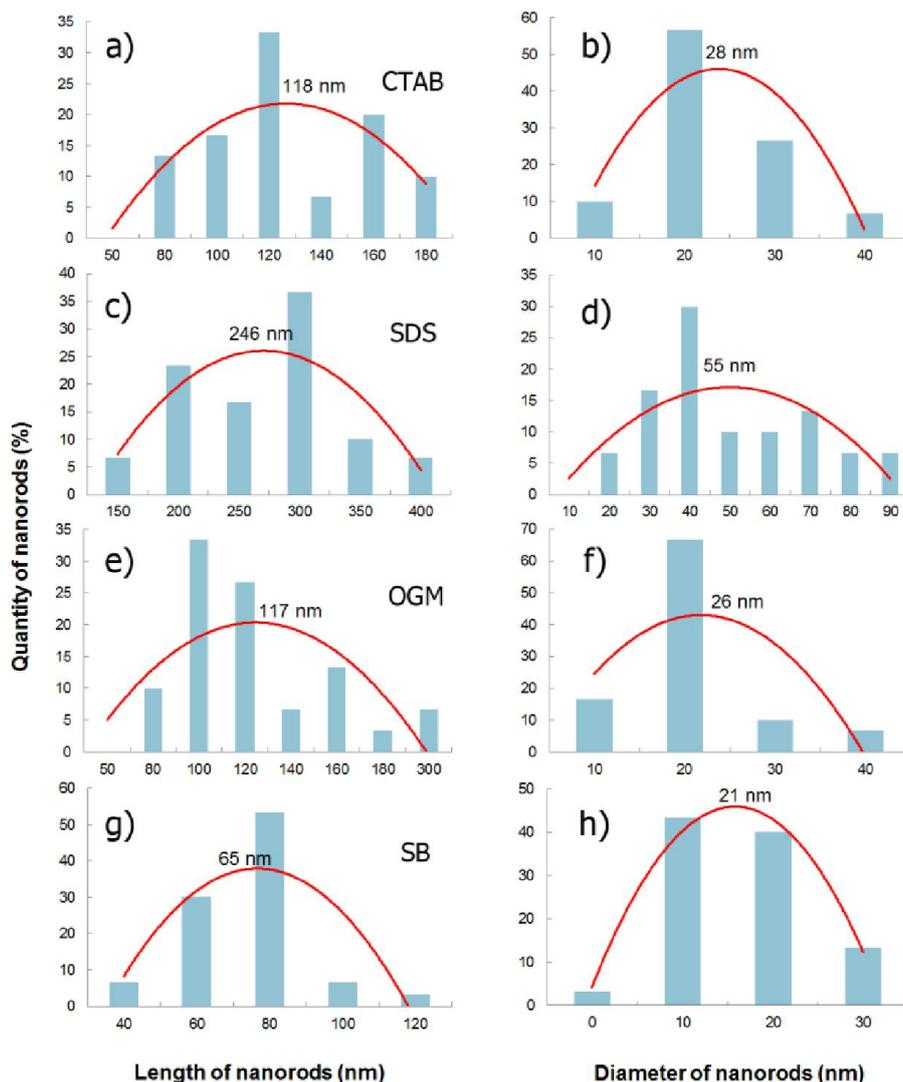
Fig. 5. Distribution of diameters and lengths of the ZnO nanorods prepared using different kinds of surfactants: (a, b) CTAB, (c, d) SDS, (e, f) OGM, (g, h) SB.
