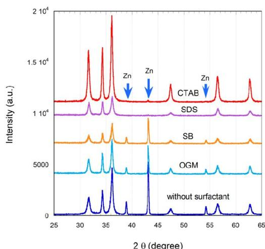
**Fig. 3.** XRD patterns of the samples produced by the pulsed plasma using zinc electrodes submerged in different surfactant solutions. The arrows denote the diffraction angles positions, where the prominent peaks belonging to metallic zinc reflect.
