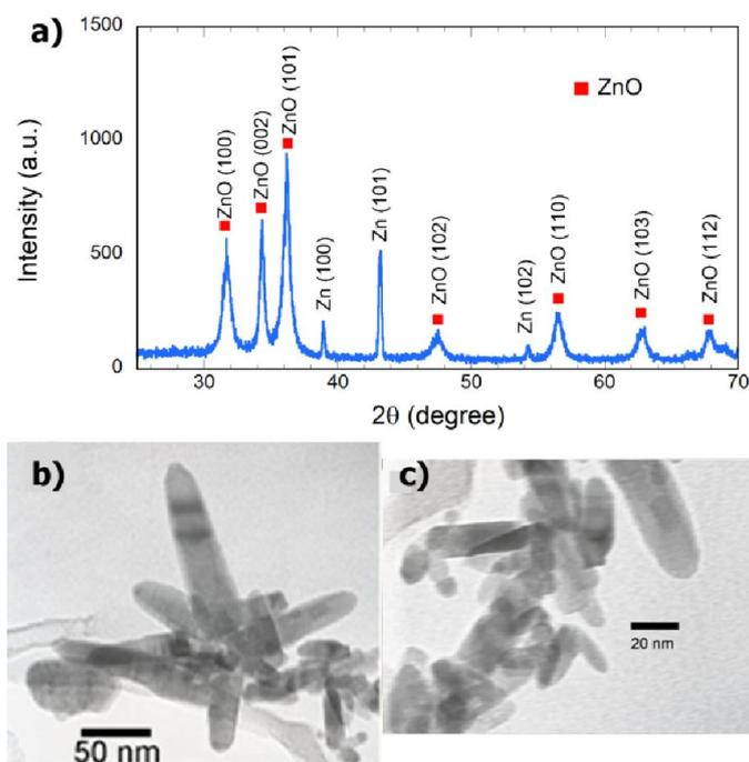
**Fig. 1.** a) XRD pattern of the synthesized sample by the pulsed plasma between two zinc electrodes submerged in water. Each peak is labeled with the identified lattice plane of ZnO or Zn. b) and c) TEM images of the synthesized sample.
