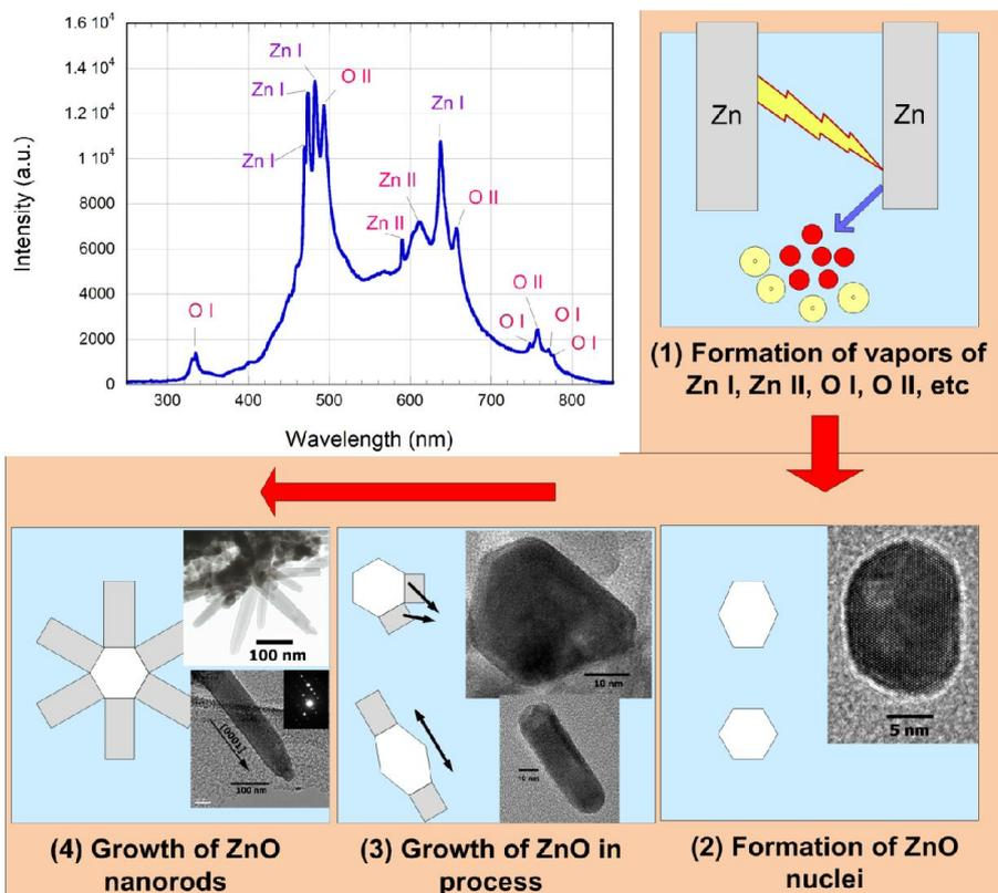
**Fig. 2.** Atomic emission spectrum of the plasma generated by the pulsed electric discharge between zinc electrodes in water and the formation pathway of the ZnO nanorods with insets of HRTEM images of the sample.
