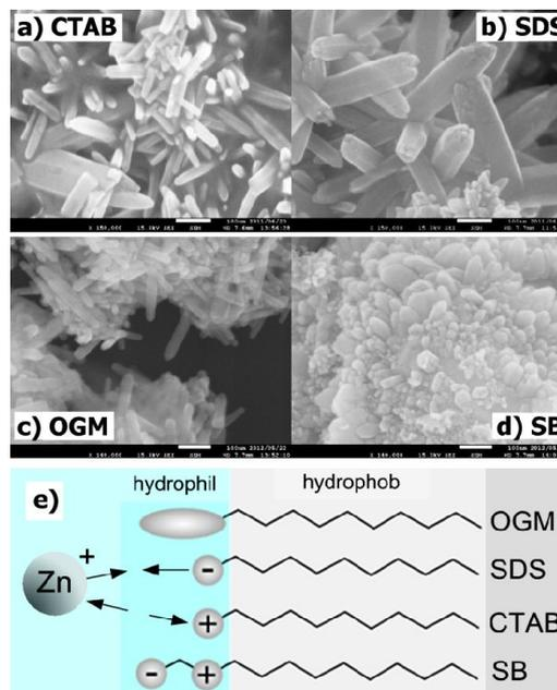
**Fig. 4.** (a-d) FE-SEM images of the produced ZnO samples by using different kinds of surfactant materials. The images were taken at similar magnification and thus the scale bars in the images are same and equal to 100 nm. e) Schematic illustration of possible interaction between the Zn ions and the surfactant materials during the formation process.
